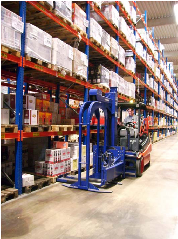
Figure 3: Current test series with the pallet turning device show, that the total pick time per warehouse worker can be reduced by 6,7%.
