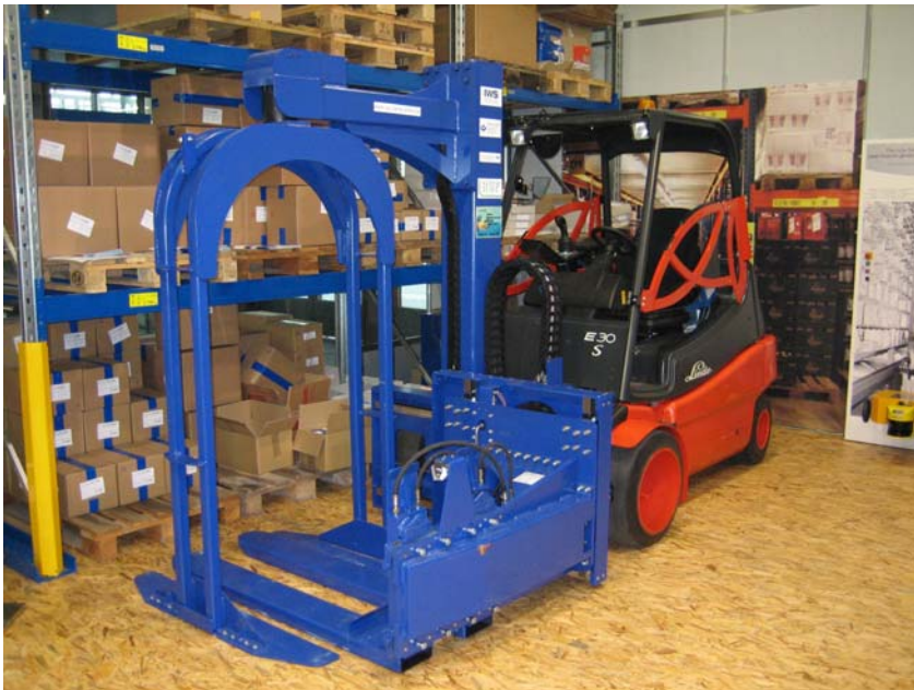
Figure 1: As attachment for lift trucks, the pallet turning device developed by IWS reduces the risks for warehouse workers of work related musculoskeletal disorders and improves productivity.
