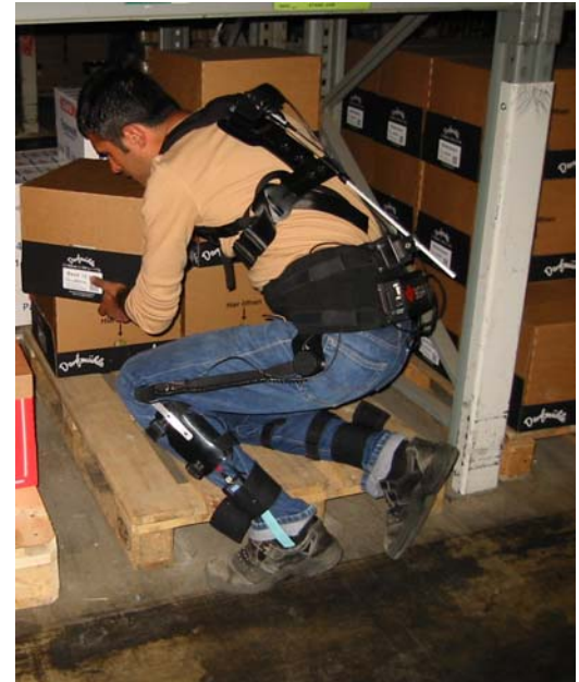
Figure 2: The test persons were equipped with the Cuela measuring system to evaluate the load of the musculoskeletal system and analyse body postures of warehouse workers.
